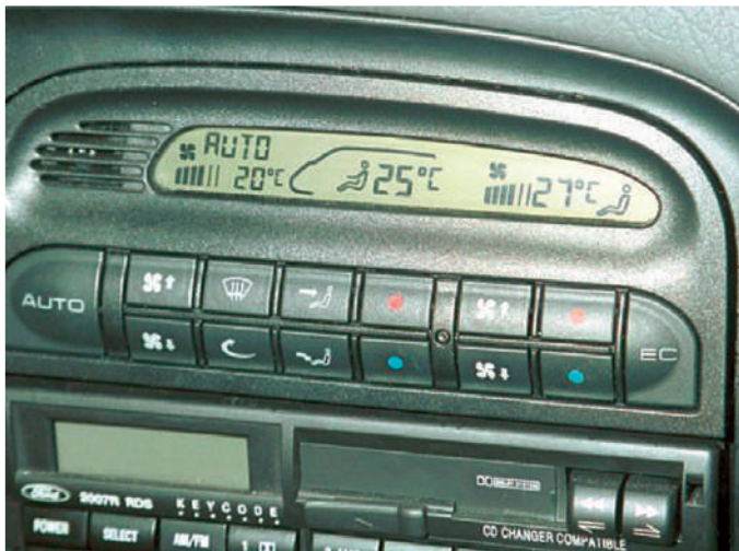
Figure 2.174 Air flow and heater controls
